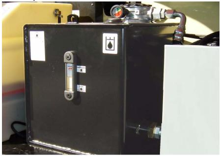
Lube Point(s) - Fill Cap Capacity -Prior to S/N 51941 - 15 gal. tank (56.7 L) S/N 51941 to present - 15.9 gal. system (56.7L) 12.4 gal. (46.9 L) to Full Mark Lube - HO
