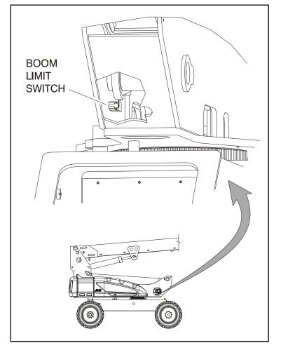
9. Boom Limit Switch - Switch operable;
