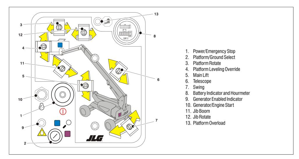
Figure 3-1. Ground Control Station
