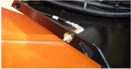
Lube Point(s) - 1 Grease Fittings Capacity - A/R Lube - MPG Interval - Every 3 months or 150 hrs of operation
