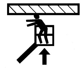
• During operation, keep all body parts inside platform railing.
