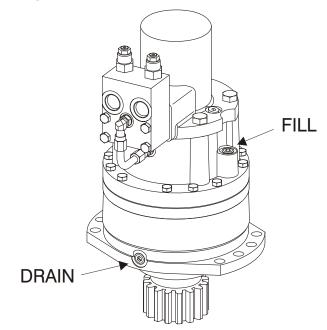
Lube Point(s) - Level/Fill Plug Capacity - 24 oz. (0.7 L) Lube - EPGL
