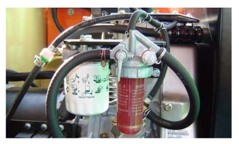
Lube Point(s) - Fill Cap Capacity - Refer to engine manual Lube - EO Interval - Check daily. Change in accordance with engine manual.
